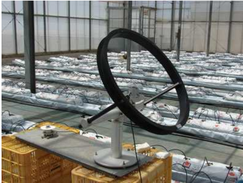
A device for measuring diffuse radiation. PHOTOS COURTESY NICOLAS CASTILLA
